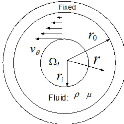
Fig. 1 Coordinate system for incompressible viscous flow between a fixed outer cylinder & a teadily rotating inner cylinder
