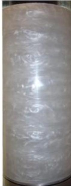
*Fig.5 Flow patterns in rotating Couette flow in Turbulent condition*
