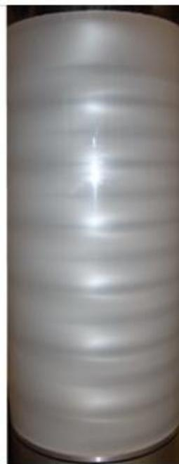
*Fig.4 Flow patterns in rotating Couette flow showing Taylor Cells*
